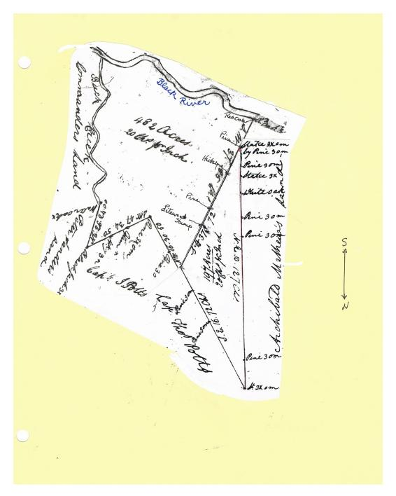
The two plats fit together thus. The surveyor marked the same trees on each plat so it is possible to line up a pine with 3x, a litewood stump, another pine, and a hickory to see how the plats fit together. The fact that the 197-acre plat does not go all the way to the river raises the question of whether there may have been a ferry landing there, but a surveyor would usually have noted it.
